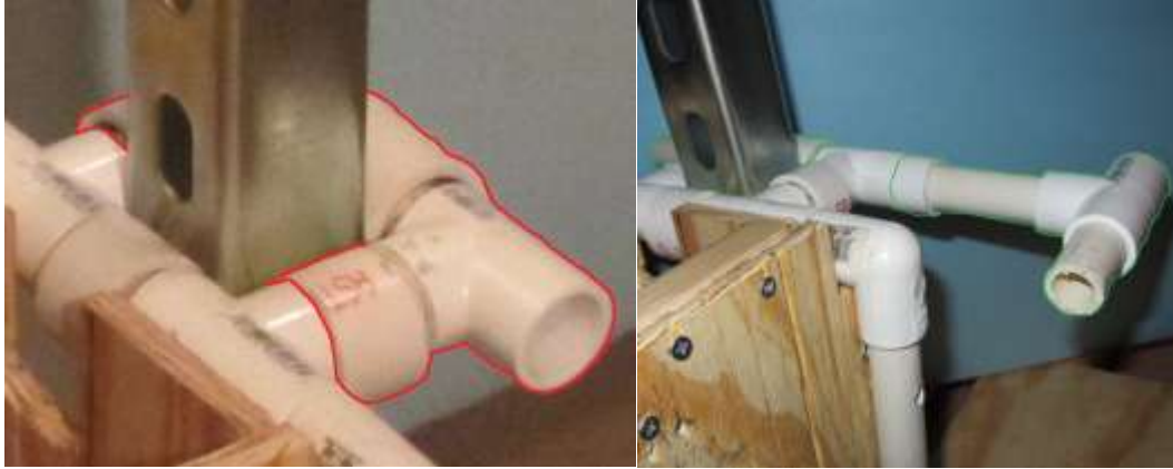
Figure 6.3 The original stabilization had a removable back (red). However, this easily fell off and wasn't the fastest to mount. The improved system had a pin that could be pulled in and out (green). It was faster, stayed on better, and could mount a piece that could hit the summit indicator.
